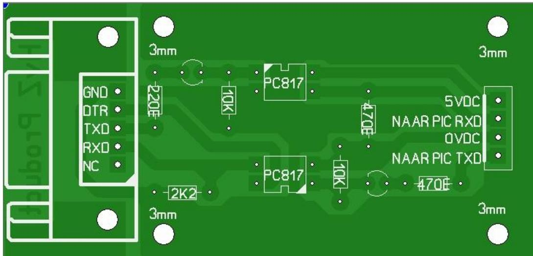
The PCB is made with Sprint-Layout 4.0, just like the rest of the PCBs that follow. On the left side of the PCB you see a 9-pin SUBD connector for the RS232 connection. On the right side of the PCB you can see the connection at the front of the controller, this is done with a four-pin connector from Molex.
