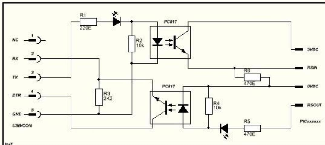
The power supply for the RX signal comes from the DTR pin, which becomes high when Profilab is active. If the RSOUT signal from the controller now goes high, then the RX pin will also go high. The TX pin in turn controls the RSIN pin on the controller. On the right side of the diagram you can see that the power is coming from the controller, in this case it is 5VDC.
