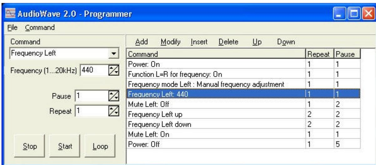
The commands from command list on the right are executed one after another. Press START to start a program. STOP immediately terminates a sequence. LOOP restarts a program, when the end of a program is reached. Make sure that AudioWave is started, before executing a program.
