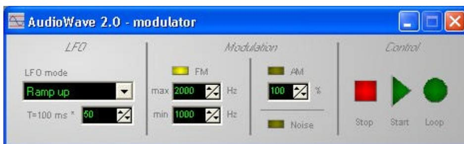
Use the modulator to produce sine signals with modulated frequency or amplitude.
